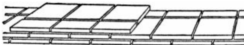
VITRUVIUS' BRICK-BOND ACCORDING TO REBER
